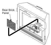
Figure 42 - Installing Rear Brick Panel
